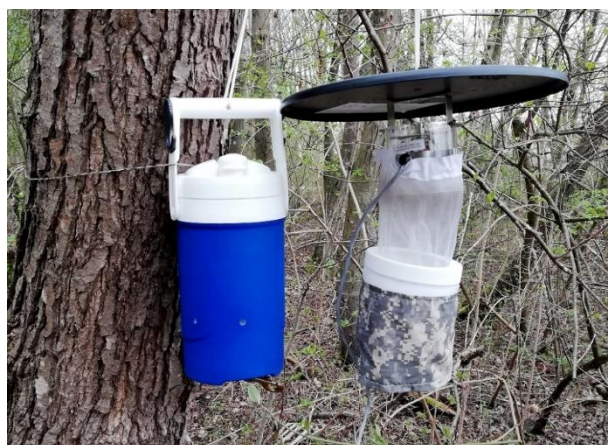
Figure 2: CDC trap with blue dry ice container (Photo: A. Gander).
